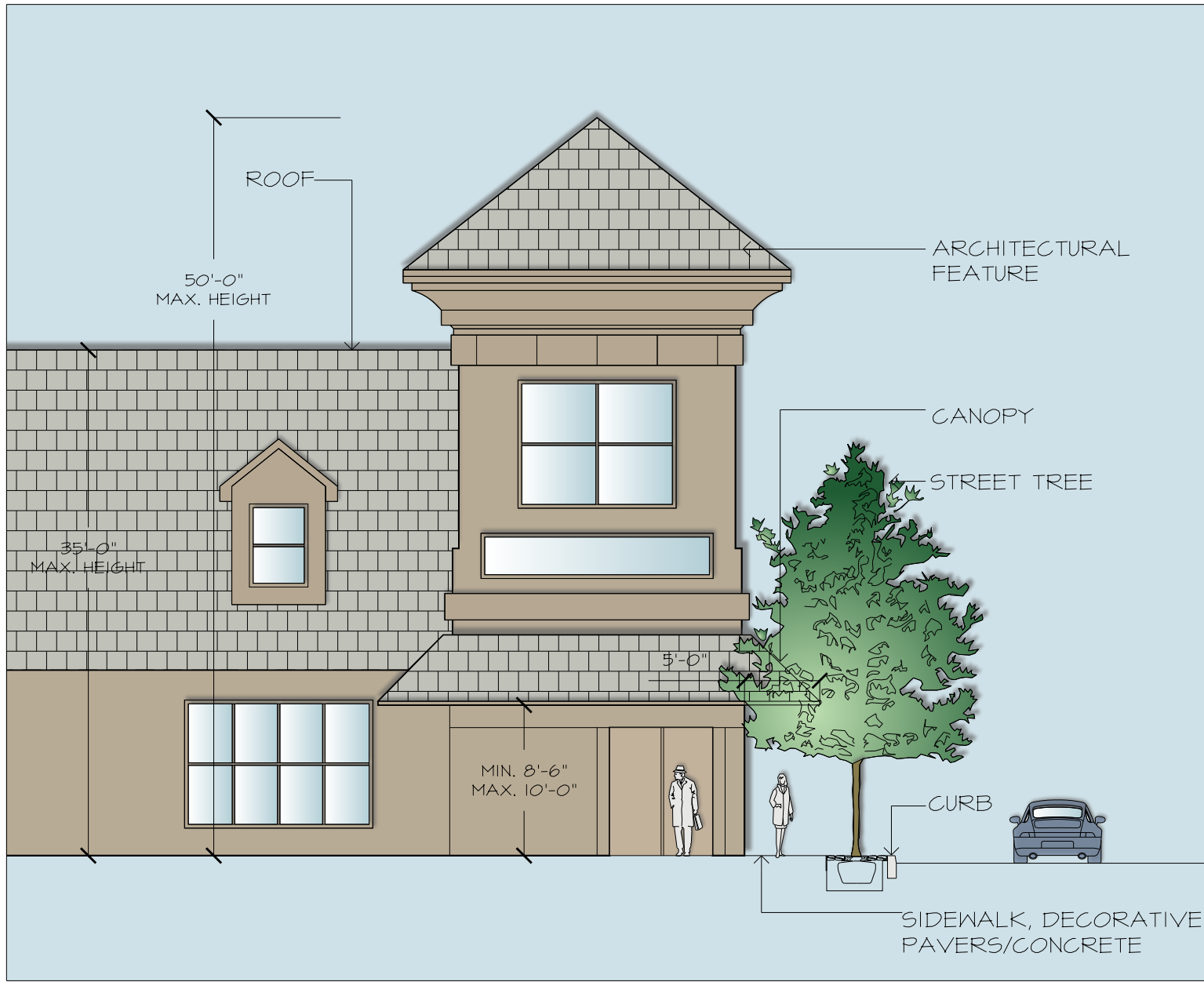
LD-2 ARCHITECTURAL & SIDEWALK SECTION SCALE: 1"=10'-0"
